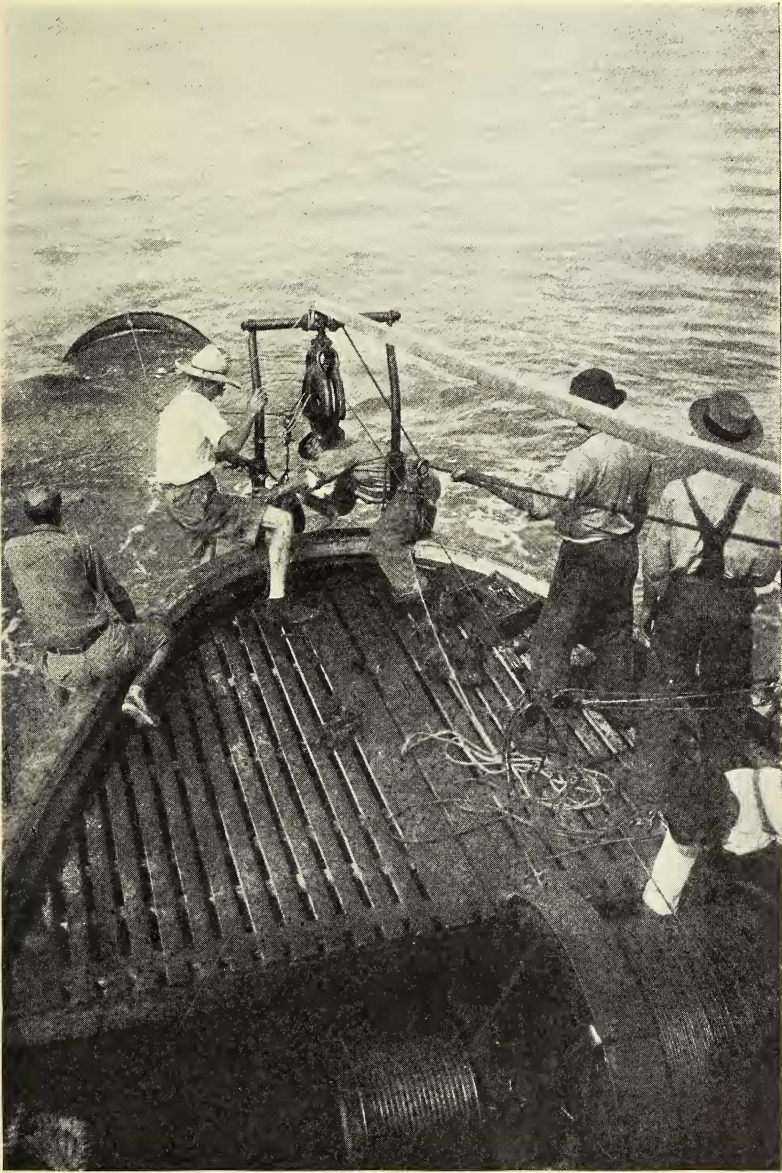
Fig. 5. Metre net, sheave, wire and winch on the aft deck of the Gladisfen .
